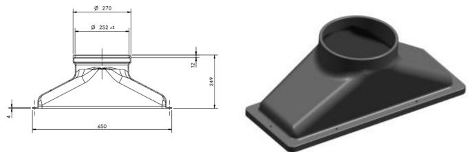
In the case of higher modulations (2100 mm and 2400 mm) there are 2 hoods distributed longitudinally, achieving a very linear sweep on the front of the sash, even improving the performance of lower modulation fume cupboards, as shown in the image below.
